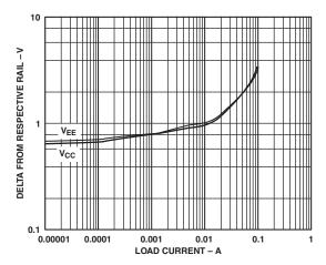
Figure 22. AD8610 Dropout from ±13 V vs. Load Current
