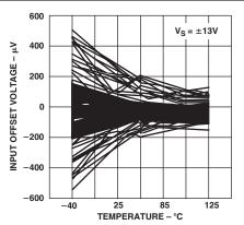
TPC 2. Input Offset Voltage vs. Temperature at ±13 V (300 Amplifiers)
