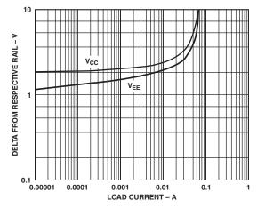
Figure 23. OPA627 Dropout from ±15 V vs. Load Current
