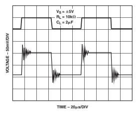
Figure 6. AD8610 Capacitive Load Drive,  $A_V = +2$
