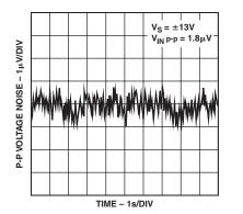
TPC 25. 0.1 Hz to 10 Hz Input Voltage Noise
