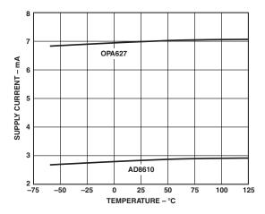
Figure 1. Supply Current vs. Temperature
