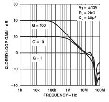
TPC 16. Closed-Loop Gain vs. Frequency
