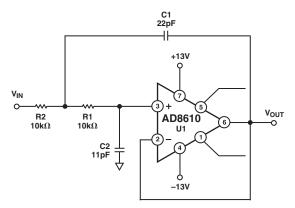
Figure 27. Second Order Low-Pass Filter
