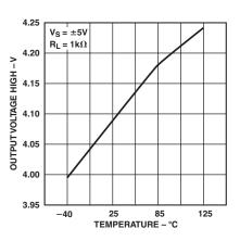
TPC 11. Output Voltage High vs. Temperature at ±5 V
