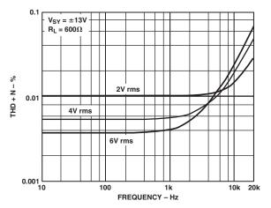
Figure 17. THD + Noise vs. Frequency
