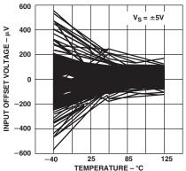
TPC 4. Input Offset Voltage vs. Temperature at ±5 V (300 Amplifiers)
