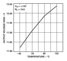
TPC 13. Output Voltage High vs. Temperature at ±13 V
