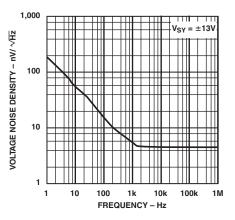
TPC 26. Input Voltage Noise vs. Frequency
