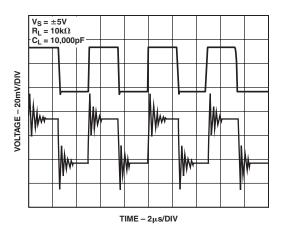
Figure 3. AD8610 Driving  $C_L = 10,000 pF$
