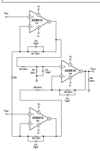
Figure 26. High-Speed Instrumentation Amplifier
