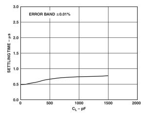
Figure 20. AD8610 Settling Time vs. Load Capacitance
