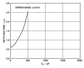
Figure 21. OPA627 Settling Time vs. Load Capacitance
