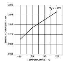
TPC 8. Supply Current vs. Temperature at ±13 V
