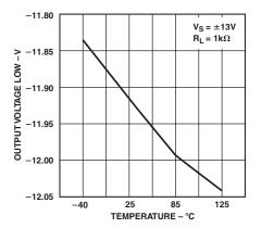
TPC 14. Output Voltage Low vs. Temperature at ±13 V
