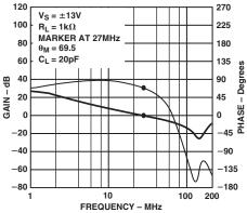
TPC 15. Open-Loop Gain and Phase vs. Frequency
