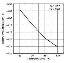
TPC 12. Output Voltage Low vs. Temperature at ±5 V
