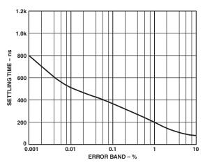
Figure 18. AD8610 Settling Time vs. Error Band
