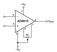
Figure 24. Offset Voltage Nulling Circuit
