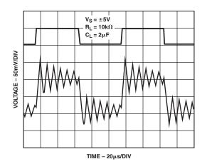
Figure 5. OPA627 Capacitive Load Drive,  $A_V = +2$
