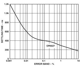
Figure 19. OPA627 Settling Time vs. Error Band
