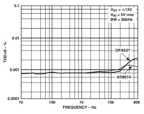
Figure 16. AD8610 vs. OPA627 THD + Noise @  $V_{CM} = 0 V$
