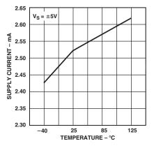
TPC 9. Supply Current vs. Temperature at ±5 V
